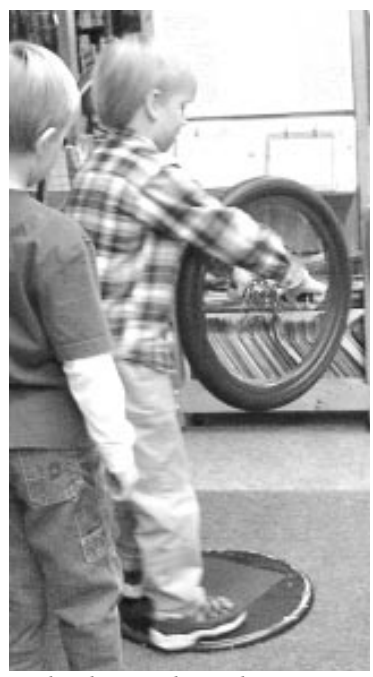
The device above demonstrates the principles of inertia and momentum. When the subject changes the plane of the spinning wheel's rotation by turning the axle, the turntable below compensates by rotating the subject.
